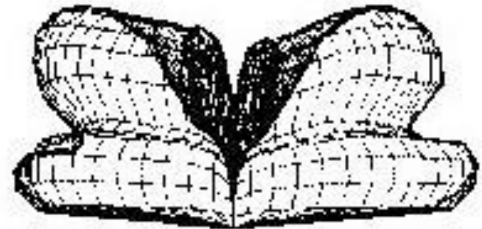
CAROLINA WINDOM 80 on 15 m with Vertical Radiator removed.
